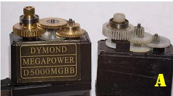
After only 15 flights, note the broken gear tooth. Yes, the servo will continue to function. And a lot of modelers are flying around with (unknowingly, of course) broken teeth on their plastic-gear servos and can't understand why their airplanes do not respond properly to their control inputs. **The message:** LOOK INSIDE YOUR SERVOS!
