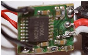
Compare that to the excellent soldering and support for the wires on the *Dymond5000* (below). Quality soldering and wire support doesn't get any better than this, and we don't care what brand you are looking at.
