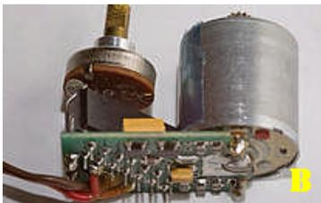
In another well-known brand servo (below B) the amplifier is soldered directly to the motor. Vibration from the rotating motor is transferred directly to the amplifier and the solder joint. We do not consider this a good thing. Note: later in the photos of the *Dymond 5000* that the motor is separated from the amplifier by wires so motor vibration is not transmitted to the amplifier.
